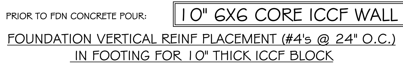
4b FDN REINF PLACEMENT/10" BLK OVERLAY/24" O.C. (b) SCALE: 3/4" = 1'-0"
